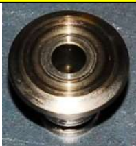
Discolouration due to poor lubrication
