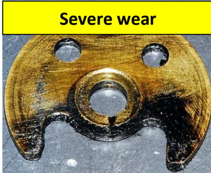
Discolouration due to poor lubrication
