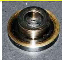
Discolouration due to poor lubrication
